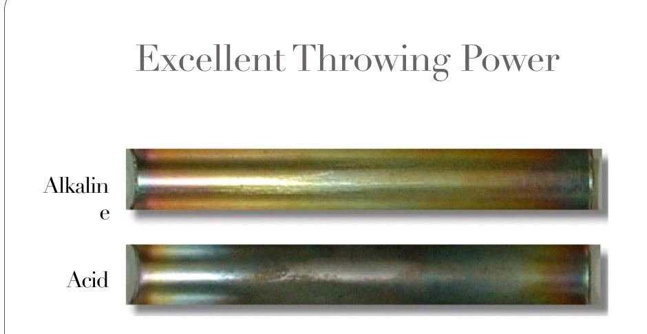
Alkaline Zinc provides significantly better coverage in extremely low current density areas as shown by this cross section view of the inside of a plated pipe.
